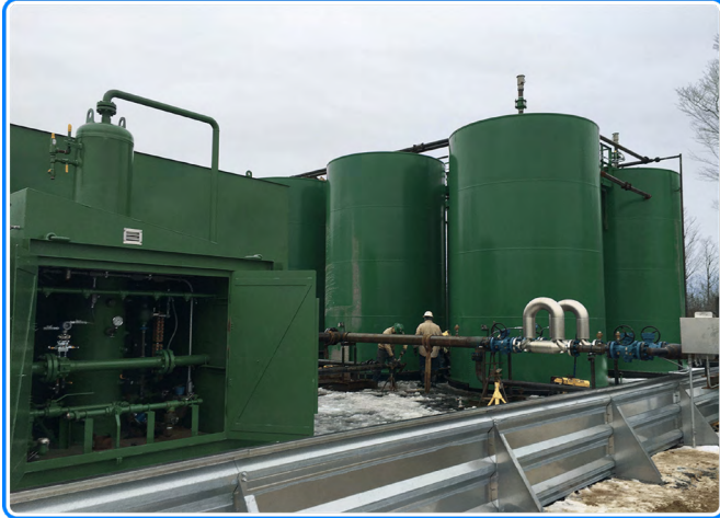
One of Seneca's gas processing units and produced water tank battery with six tanks, where gas and water are separated and measured before sending the gas into the gathering system.
