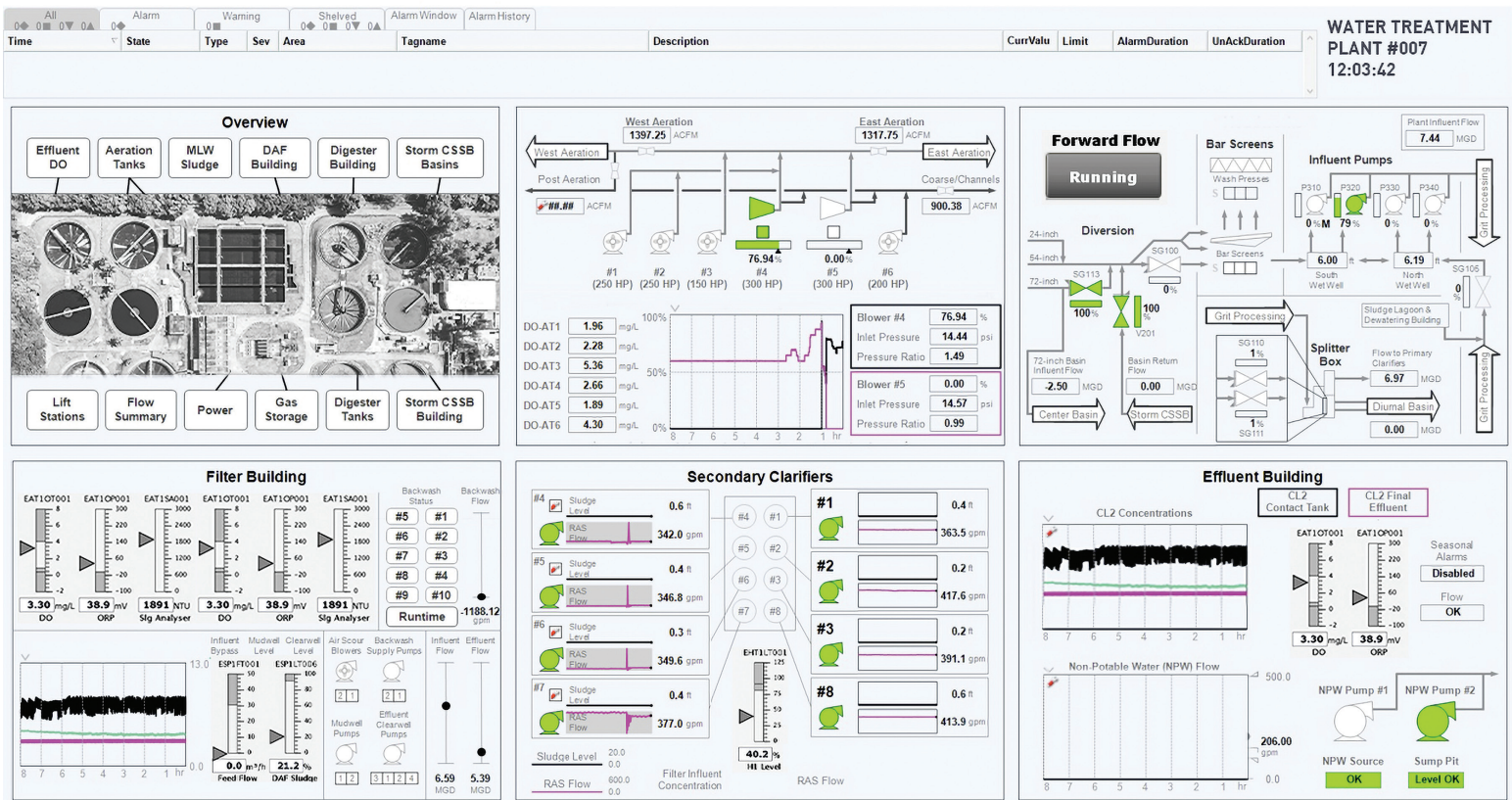
FIGURE 1: Not only can OPC UA be used to relay the real-time values like sensor readings to SCADA HMI screens across vendors; it can also relay alarm conditions that SCADA builds on top of those variables, so that dangerous or costly deviations can be quickly identified and addressed. Courtesy: SmartSights
