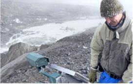
Working with Auckland-based Industrial Interface Company, a WIN-911 Solutions Provider and others, the Eastern Ruapehu Lahar Alarm and Warning System, or ERLAWS was developed. ERLAWS consists of three sites at which various geophone and water level sensors are located. These sites include Crater Lake, the New Zealand Alpine Club hut and near the Tukino ski field.
